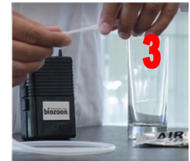
Push the other end of the tubing onto the thin end of the disposable pipette
