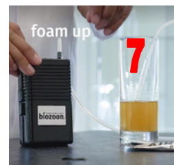
Switch on the air pump and insert the pipette into the liquid
